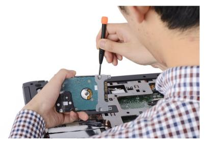
Fig. 2.2.18: Upgrading HDD
